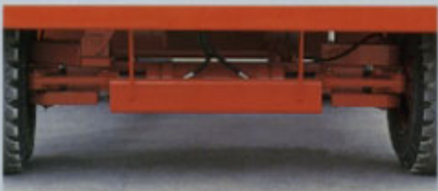
Single "double acting" steer cylinder
