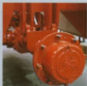
Oil cooled wet disc brakes
